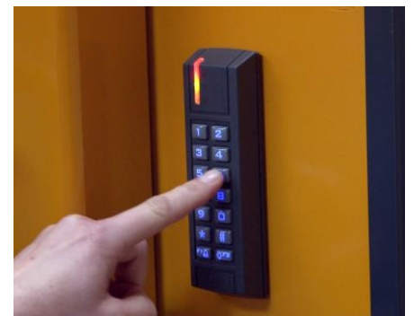
A digital auto lock will prevent unauthorized users from running the baler without a 4-digit code.
