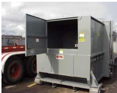
Large rear door with low feed height for safety
