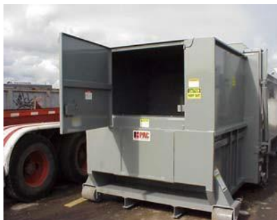
Large rear door with low feed height for safety
