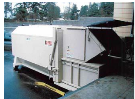
Rear fed enclosure using a hydraulically raised door and an overhang for added employee safety
