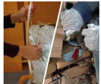
You can use either plastic strapping or baling wire to tie the finished bales.
