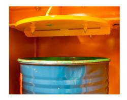
Spikes mounted underneath the press plate puncture the drum and remove air.
