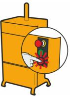
Press the lit orange finish indicator button so the platen goes back to the top position.
