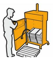
The baler must only be operated by one person. Only the operator should be in the vicinity of the baler when ejection is being performed. See chapter 6, Installation, Clearances and working area.
