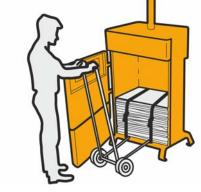
Open the doors and lift out the bale with the bale wagon, as shown in the illustration below.
