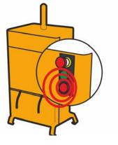
The platen will go down and park on top of the bale. The orange finish indicator button now starts to flash.
