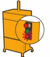
When the orange finish indicator button lights/blinks, the bale has reached its maximum and the platen parks on top of the bale.
