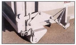
KP1SC's feature a heavy-duty single ratchet latch system which pulls the door tightly and evenly against the door seal. K-PAC's innovative latching system features an adjustable stop to prevent over compression and damage to the door seal... resulting in longer seal life and less downtime for seal replacement.
