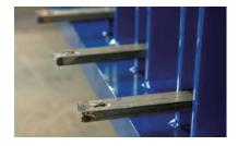
The H60 features an industry first Automatic Wire Feeder, eliminating the use of wire guides, which is the number one complaint for closed-door horizontal balers. This Harmony Enterprises patented technology cuts tying time by over 50% thus lowering your labor costs.
